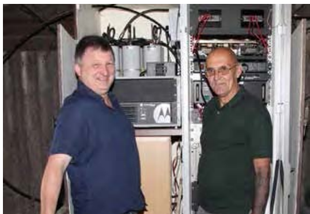
Michael, G1XCC and Mick, MOLEV with the new repeater. The cabinet also contains 23cm, 2m and 6m boxes.
